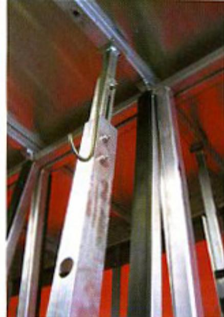
The space-gaining ledgeboard remedies space organization problems in body units by lifting glass sheets to free up space underneath for storage of aluminum framing and other materials. The extended hook of the easy-release pole helps to anchor loads down and facilitates removal from the socket.
